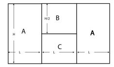
In comsol, solve the steady state conduction problem for a set temperature difference on the left and right boundaries. Compute the total heat flow with Comsol and define the overall effective resistance as the ratio of the total temperature difference to the total heat flow. Compare the comsol result to the simple circuit analogy solution. Try the following sets of parameters;
